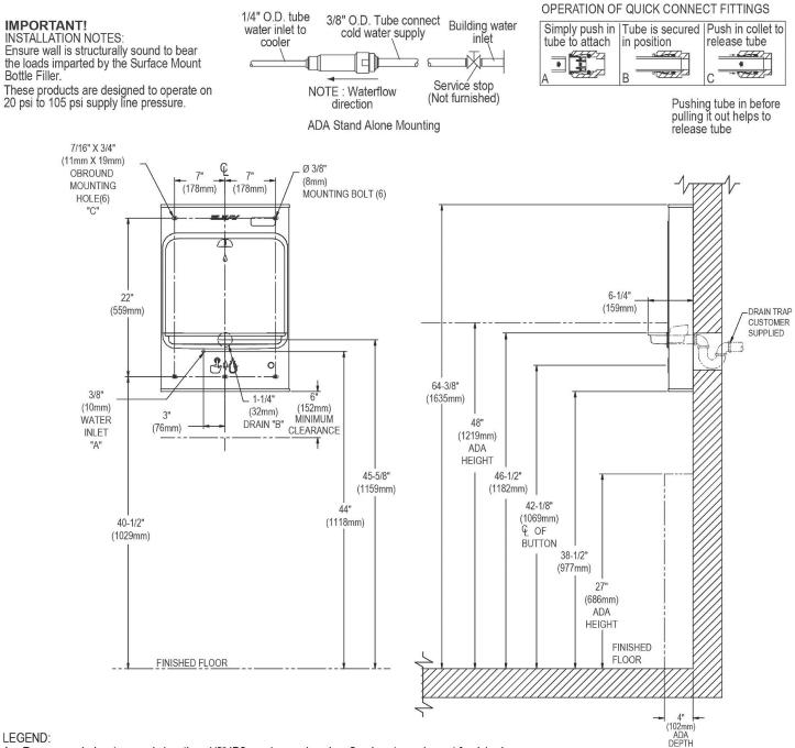
A = Recommended water supply location; 1/2" IPS maximum pipe size. Service stop valve not furnished.
