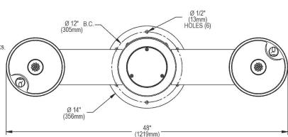
**FRONT VIEW** SIDE VIEWS **BACK VIEW** Ø 10" (254mm) (76mm) 14-9/16" (371mm) 0 44" (1118mm) 64" (1626mm)  $(\odot)$ 34-11/16" (881mm) ORIFICE HEIGHT 0 29-13/16" (757mm) ORIFICE \_\_\_ 19" (483mm) B. **HEIGHT** C 19" (483mm) 33-5/16" (846mm) 30" (762mm) 1-1/2" DRAIN 28-7/16" (723mm) \*27" (686mm) 22-1/8" (562mm) 7-5/16" 8" (203mm) (202mm) FINISHED FLOOR
